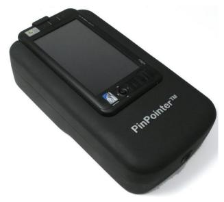
The *PinPointer™* packs a full-featured Raman spectroscopy system in a remarkably affordable true handheld format. The lightweight unit is controlled by a pocket-size Windows® computer and features easy-to-use *ID-find™* software that provides one-touch identification of unknown substances by immediate comparison of a measured spectrum to the on-board Raman spectral library.
